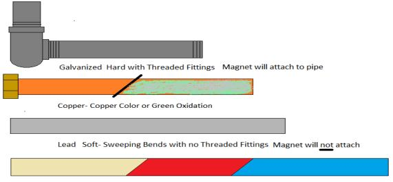
Plastic / PVC / PEX Glued Joints, Crimped Fittings. White, Tan, Blue, Red
